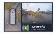
By longer pressing the **MODE**-button (ca. 3 seconds) you can switch to fullscreen mode. Here you can choose front or rear cam in fullscreen. By pressing the **MODE**-button shortly you can switch from front to rear and back. Holding the **MODE**-button again for ca. 3 seconds will bring you back to combined 360° view.
