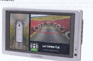
OMNIVUE-system starts automatically bei igniting your vehicle. If you've connected a further camera to your CM-708 display you can switch by pressing the (M) Modebutton.
