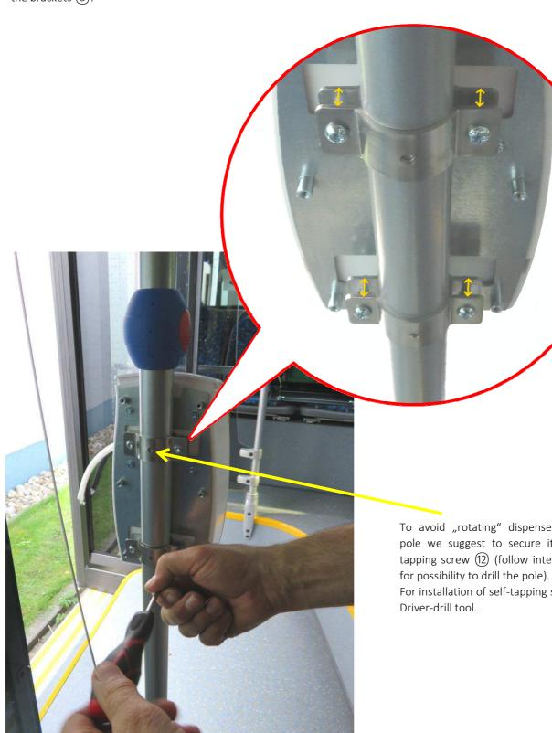
To avoid "rotating" dispenser on the pole we suggest to secure it by selftapping screw (12) (follow internal rules
