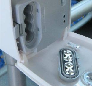
Insert 4 pcs new AA alkaline batteries so that the polarity of the inserted batteries matches the polarity markings on the dispenser control unit body.
