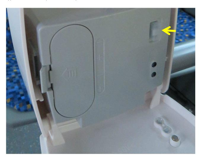
Make several "sprays" by repeatedly placing your hands under the dispenser to expel air from the disinfectant transport tubes in the dispenser control unit.
